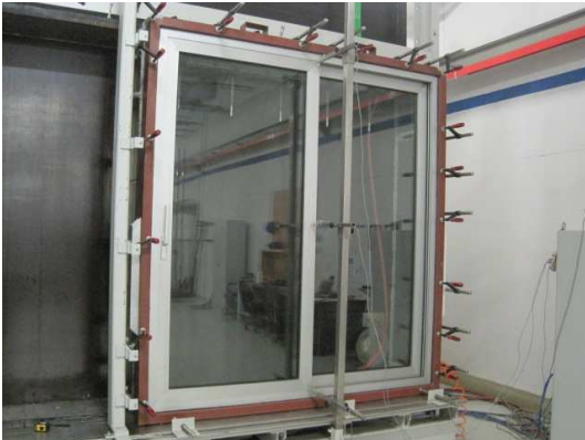
Picture Test setup measurement of deflection
