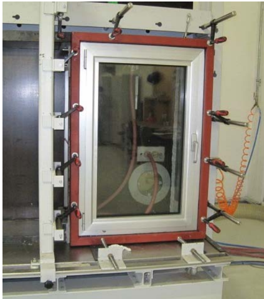
Picture View of test specimen on window test rig Window closed
